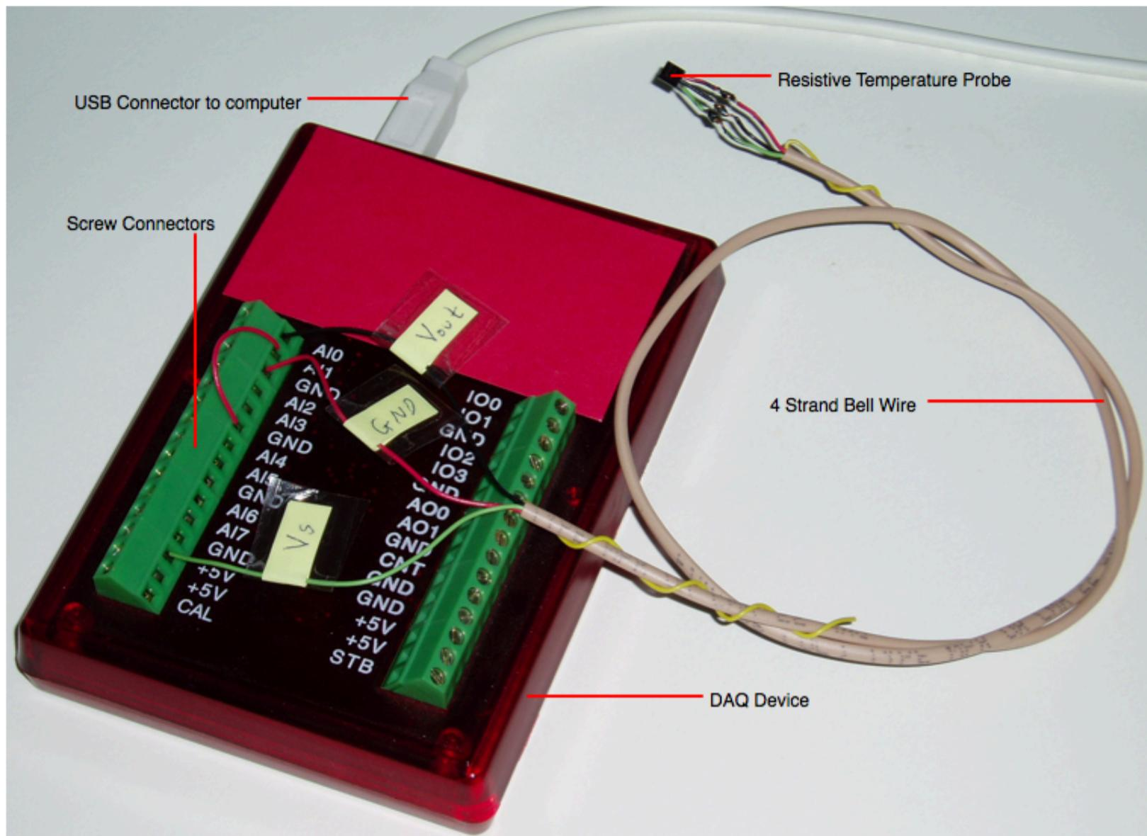
The sensor produces a voltage proportional to heat. That voltage is connected to the AI0 connector of the DAQ device. That voltage has to be compared to some other voltage, which in this case is a ground voltage. Hence, the AI1 connector is wired to the ground connector on the DAQ device.
