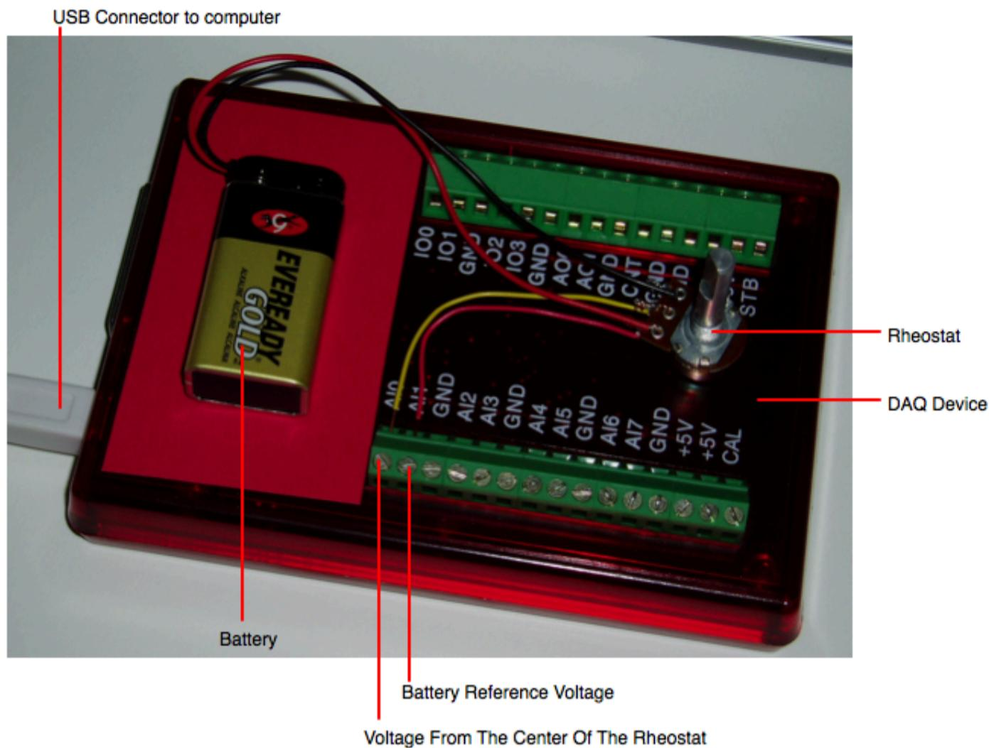
By turning the rheostat knob you change the voltage and thus change the value of the curve shown on the DAQ Plot graph.
