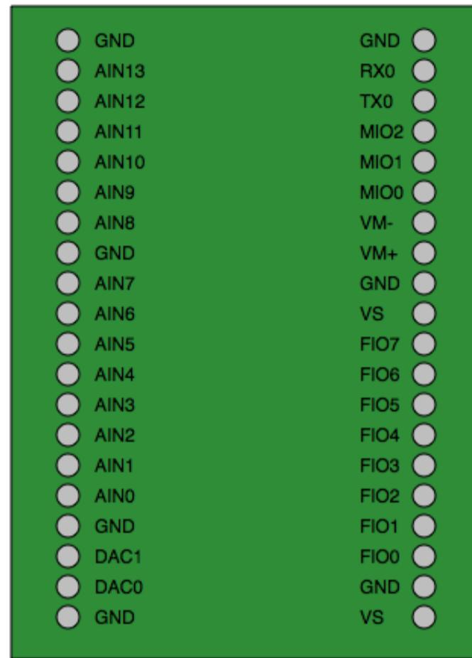
Terminals AI0-AI13 are the 14 analog input channels. DAC0 and DAC1 are the two analog output feedback channels. FIO0-FIO7 are the 8 digital output channels.
